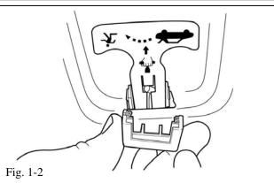
(b) Remove the trim bezel for the emergency trunk release and then remove the handle for the release cable. The trim bezel can be unsnapped by hand (Fig. 1-2).
