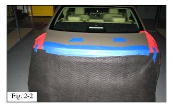
(c) Apply masking tape to the trunk lid surface in the areas of the hole locations (Fig. 2-2).
