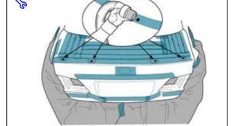
(j) Vacuum the surface of the trunk lid and the surrounding drilled areas, then remove the masking tape (Fig. 2-5).
