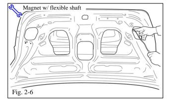
(k) Open the trunk lid and use a magnet with a flexible shaft to remove any remaining metal chips from the drilling process (Fig. 2-6).
