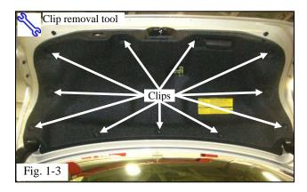
(c) Remove the 11 black clips from the trunk inner panel and retain them for reinstallation (Fig. 1-3).
